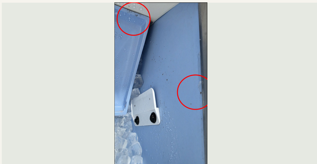
Mould build-up inside the ice maker. (Source p. 19)
